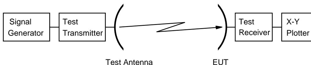
**Figure 3: Test arrangement - antenna receive pattern measurement**
